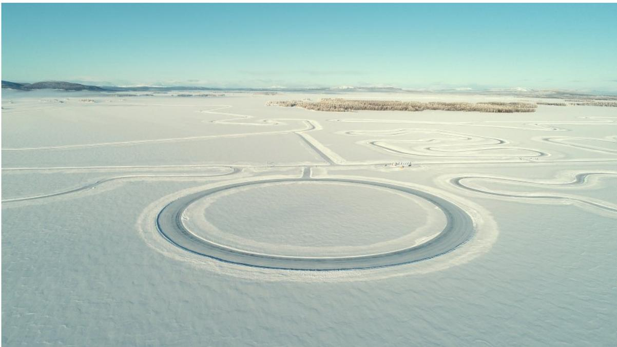
As their name suggests, by means of a radius of constant curvature and a width of 20 meters, these two circles will allow you to learn to maintain a constant drift, with more or less angle. The diameter of the smallest one is 250m while the biggest is 350m !
